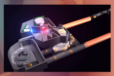
passes through a dual-stage filter. The first stage removes dust and dirt from the air sample before it enters the laser detection chamber. The second (ultra-fine) stage provides an additional clean air supply to keep the detector's optical surfaces free from contamination, ensuring stable calibration and long detector life.
